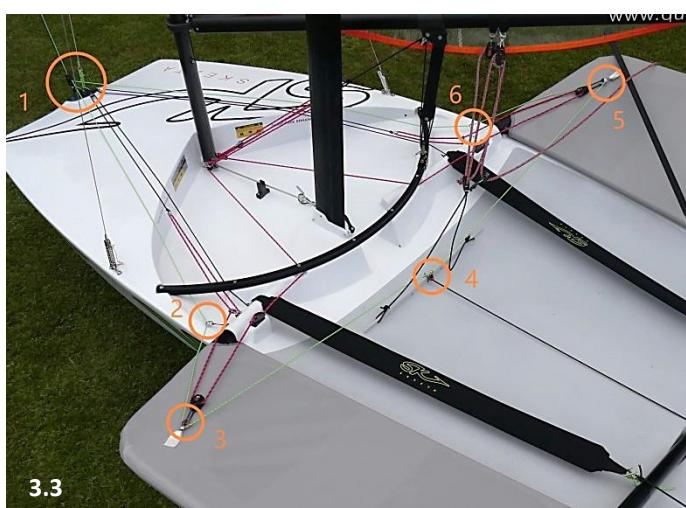
The wand is now ready for use, Pull the cord to raise or lower the wand. This changes the ride height while sailing. Always start with the wand raised until you are ready to fly. If you need to stop foiling or slow down quickly and safely, raise the wand to lower the boat to the water surface.
