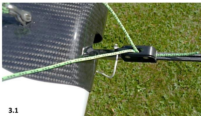
First off, insert the wand inside the wand tube assembly, ensuring the rope is sitting in the groove at the back of the wand. (pic 3.1)
