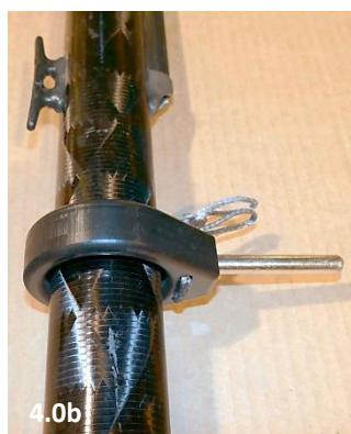
Slide the aft end of the boom into the clew loop on the sail (4.0a), then slide the forward end of the boom onto the gooseneck pin at the tack of the sail (pic 4.0b).
