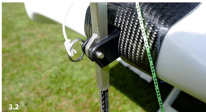
When finishing the closed loop, it is best to push the wand down the tube, so the top of the wand is just below the entry and exit slot for the rope. Then insert the tail of the wand rope in and push the wand up. Insert the tail of the wand rope in the top wand hole and tie a knot. There is extra tail for adjustment if need be.
