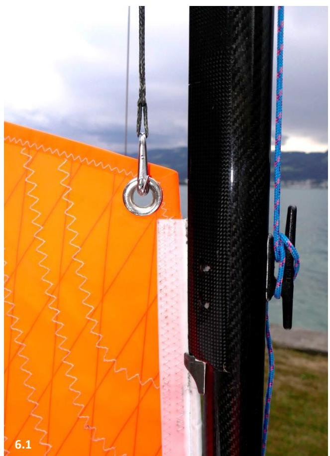
Attach the halyard hoist shackle to the top of the sail and feed the luff up the sail track on the back of the mast (pic 6.1)
