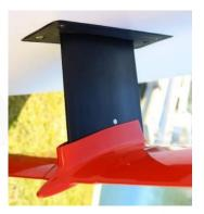
3. When leaving the shore, use the foil clamp to hold the daggerboard at the appropriate height to safely leave the shore.
