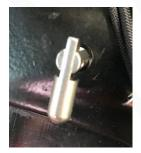
6. The excess rope can be inserted into the groove in the end of the tiller.
