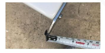
2. Walk to the head of the mast and measure the distance to the top of the carbon mast (not the plastic head fitting).
