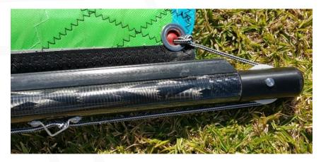
To adjust the sail hoist height, position the knot along the cord within the locking ball.
