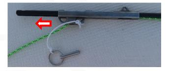
3. Push the wand tube assembly into the groove on the bow mechanism and push the fast pin into the holes to connect both components together.
