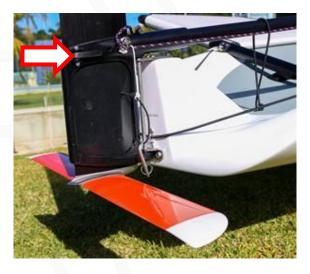
4. Insert the pull-down rope into the hole on the top of the rudder and tie a knot. The rudder is pulled down into place after leaving the shore using this rope.
