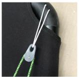
5. Return the cord to the wand tube and thread the cord up the wand as shown. When finishing the closed loop, it is best to push the wand down the tube, so the top of the wand is just below the entry and exit slot for the rope. Then insert the tail of the wand rope in and push the wand up.
