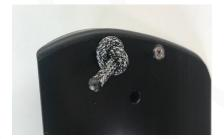
5. To lock the rudder into place, pull the retaining toggle pin over the top of the rudder and onto the opposite side of the rudder box. Insert it through the rudder box and rudder hole. Make sure the toggle pin nose drops to be engaged properly.
