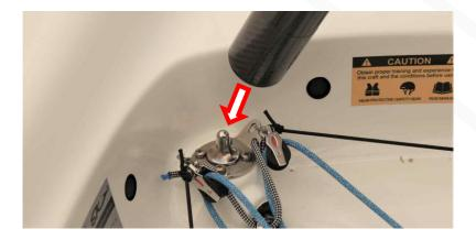
5. Support the mast and attach the remaining stay.
