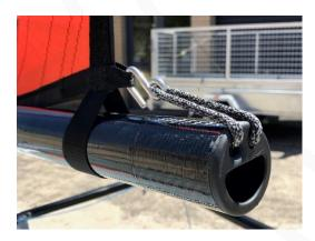
2. On the topside of the boom there is a v-cleat, the rope passes through this and can be adjusted as necessary.
