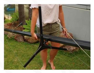
1. To attach the spreader onto the mast; Insert the spreader base into the attachment on the mast base and insert the 1/4" clevis pin and put the ring on to prevent the clevis pin falling out.
