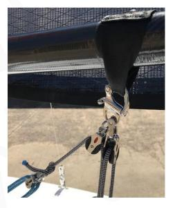
When the vang is applied, the luff is free to move down the mast, which applies both luff and leach tension at the same time. This greatly simplifies the controls and gives more time to concentrate on sailing the boat.
