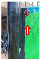
3. When the sail is fully raised, insert the knot into the halyard lock on the front side of the mast.
