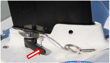
3. When leaving the shore, use the foil clamp to hold the daggerboard at the appropriate height to safely leave the shore. Once in deep water, open the clamp and push the daggerboard fully down and insert the retaining pin through the hole in the foil case and daggerboard. Pull the shock cord attached to the retaining pin over the top of the daggerboard and over the other end of the retaining pin.
