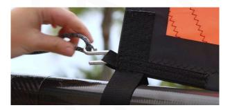
2. Insert the yoke end into the webbing loop on the tack of the sail and clip the yoke onto the mast. Ensure the webbing is positioned in front of the knob.
