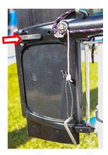
2. Attach the horizontal foil by aligning the pins and pushing it up into place.
