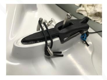
4. Once in deep water, open the clamp and push the daggerboard fully down and insert the retaining pin through the hole in the foil case and daggerboard. Pull the shock cord attached to the retaining pin over the rudder and over the other end of the retaining pin.
